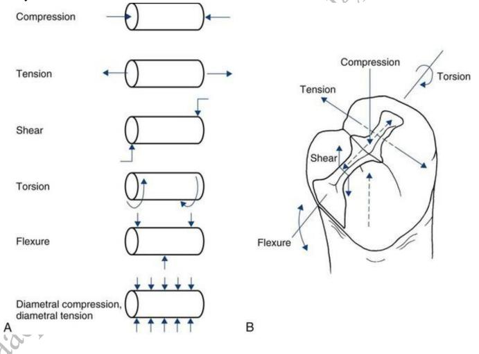
• When external force or load is applied to a material the phenomena of strain occurs; i.e. the change in the dimensions of the material.
