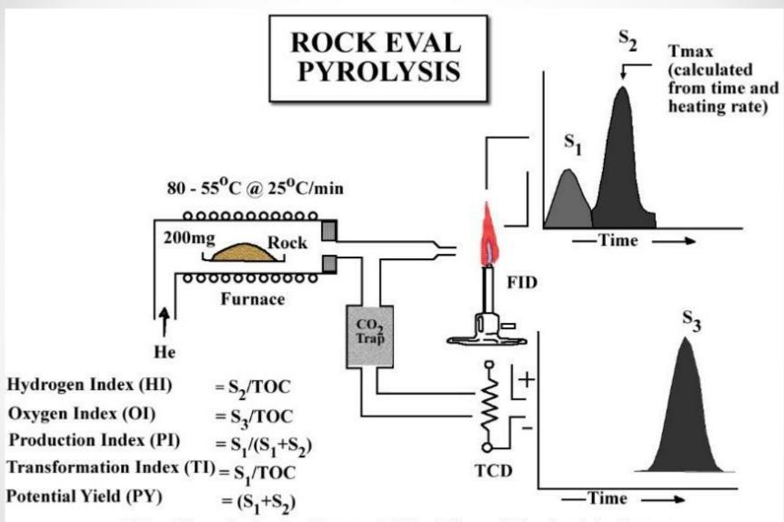
FID = Flame Ionization Detector TCD = Thermal Conductivity Detector
